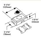
Furnished with 1/2" (12.7mm) rubber stem. Designed to accept modular connecting blocks within the fitting. Nonmetallic cover has 1500 and 2600 Series Raceway twistouts on both ends and both sides. Two 1500WC Wire Clips included. Not UL Listed. Gray finish.
