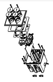
Includes dual-gang box, one 15A tamper-resistant duplex receptacle, 106 adapter with four openings for communication devices, and nickel cover with four screw plugs. For hole cut dimensions, see installation instructions sheet. Box Dimensions: 3 1/4" W x 3 3/4" L x 3 7/8" D (83mm W x 95mm L x 98mm D) Device Plate: 4 7/8" W x 5 1/16" L (124mm W x 129mm L).
