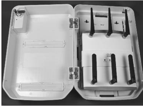
Interior of NME1250AP with wireless access point (sold separately) installed.
