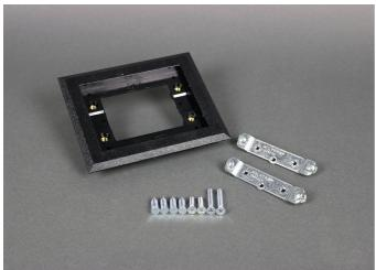
One-gang nonmetallic carpet flange. Accepts a 6A communication adapter (CM-MAB), and Ortronics MAB3S2 and MAB6TJ adapters. NOTE: Brass covers and flanges are not interchangeable with aluminum or nonmetallic covers and flanges. Nonmetallic covers are interchangeable with aluminum flanges.
