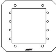
**Device Mounting Plate** – Two-gang device plate that will accept up to four (4) Extron® Electronics AAP style plates. 8AAP takes up 2 of the four (4) gangs in the center compartment. Devices supplied by others.
