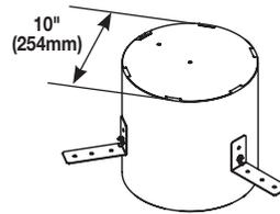
**Pre-Pour Sleeve** – Nonmetallic sleeve attaches to structural decking or plywood base and maintains a 10"-10 1/8" (254mm - 257mm) cast in hole. Includes three (3) attachment lugs, three (3) thumb screws and two (2) end caps.
