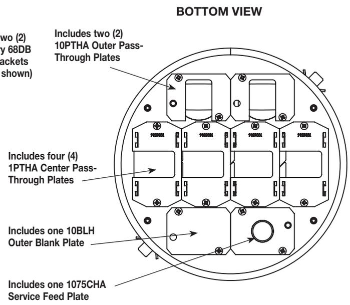
**NOTE:** For more information on Device Plates and Bottom Feed Plates and on the additional options available, see the Device Plates and Bottom Feed Plates sections found later in this document.
