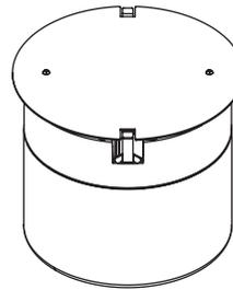
**Abandonment Plug Assembly** – Complete abandonment plug assembly for 10" opening. Assembly includes intumescent fire stop material to maintain a 2-hour fire rating of the floor.
