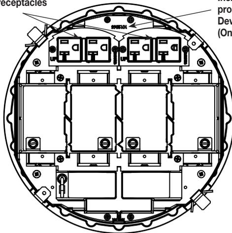
Includes two (2) proprietary 68DB Device Brackets (Only one shown)
