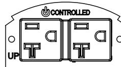
**Controlled Receptacle** – 20A proprietary TR duplex receptacle marked with controlled receptacle marking.
