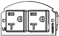
**20Amp Duplex Receptacles** – Two (2) proprietary TR 20AMP duplex power receptacles with mounting plates and 25' leads. Designed to fit in either of the two side compartments in the 6ATC, 8ATC and 10ATC Series Poke-Thru Devices. Receptacle can be wired as a standard or isolated ground device.
