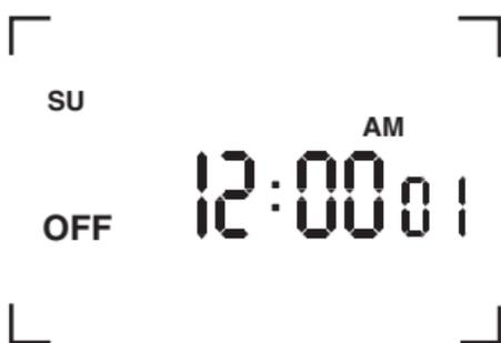
NOTE: Once you select and ENTER the above format (either AM/PM or 24 hour military), you cannot alter it without removing all power to the unit by disconnecting the battery and line power.
