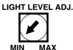
**IMPORTANT:** The potentiometer allows you to adjust a turn ON ranging from 1 to 100 footcandles. OFF will be 3 times the ratio of the ON foot candle level (see example "B" below).
