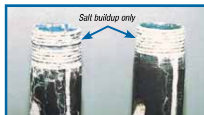
Examples of Hot-Dip Galvanized Threads after 42-day salt-fog test
